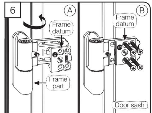
(A) Locate the sash part onto the hinge pin and rotate until against the sash. Now fit the sash datum onto sash part locating the pins into the 4mm holes on the sash. (B) Using appropriate screws, fasten sash part to your door sash.
