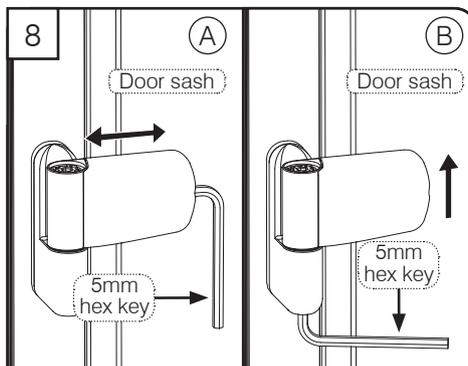
(A) **Lateral adjustment:** Remove lid cap and using 5mm hex key adjust up to  $\pm 5$ mm. (B) **Vertical adjustment:** Remove frame end cap and using 5mm hex key adjust up to  $+ 4$ mm.
