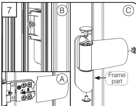
(A) With all the sash parts fitted, slide the sash lid in situ. (B) Open the door to gain access to the lid screw and tighten the lid screw. (C) Fit sash end cap, bottom frame end cap and lid cap.
