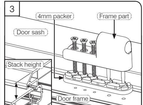
With the holes drilled, align the frame part with the pins to the bottom of the door. For 21mm or greater stack heights, fit the supplied 4mm packer. Using appropriate screws, fasten frame part to your door frame.
