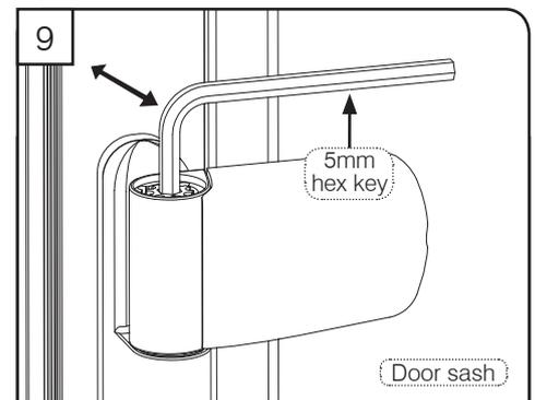
**Compression adjustment:** Remove sash bush cap and using 5mm hex key adjust up to  $\pm 1$ mm.
