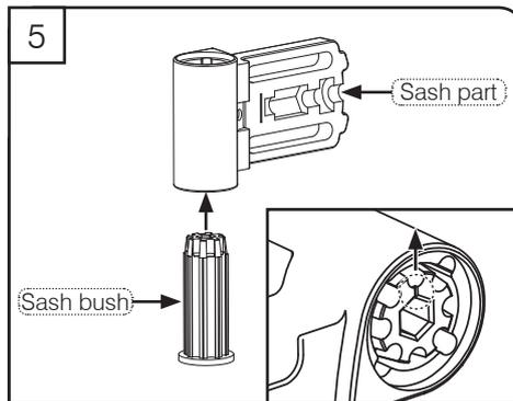
If the sash bush is not fitted, fit the sash bush with the mark pointing to the top of the sash part. As standard the sash bush should be fitted with the mark to the upwards position.
