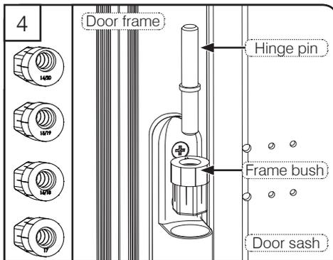
Depending on stack height, select the appropriate frame bush. By turning the bush 180° each bush gives two height options, except for 17mm version. Fit frame bush in the correct orientation with the hinge pin.
