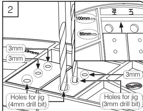
Ensure jig is set to 85 or 100mm to suit hinge. **Sash drilling:** Ensure the jig doesn't move position. For datum pegs, use a 4mm drill bit to drill the front 2 holes from frame side. For screws use a 3mm drill bit to drill the 4 remaining holes.
