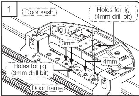
Centralise door sash within frame at correct coverage. Place jig tightly up to the sash in the desired location. Ensure correct handing of jig, LH or RH should read from left to right. **Frame drilling:** For hinge pins use a 4mm drill bit to drill the first 2 holes from bottom of door. For screws, use a 3mm drill bit on the next 3 holes.
